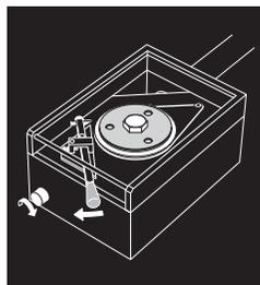
Be careful when bevelling in order that the CD is not damaged. Only when shavings are no longer produced should the moveable arm be allowed to return to its starting position.
