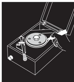
When the colouring has dried, remove the knurl by turning anti-clockwise and remove the CD carefully.
