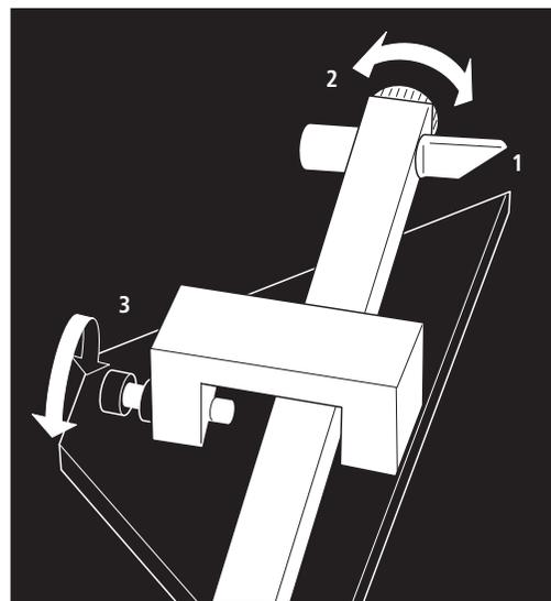
Move the moveable arm as far as possible to the left. Fix the burin in position by tightening the holding screw (clockwise turn). Here it is sufficient to use natural hand force, no excessive force should be used.
